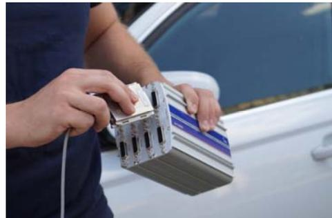
However, recently, I have noticed a stronger interest in the imc CRONOS*flex* systems. The modular and reconfigurable design allows different modules to be combined together at any time and to be spatially distributed. Furthermore, the click mechanism attracts customers – a very easy way to create your customized solution.
