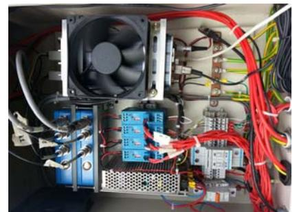
Acquisition system layout, showing imc C-SERIES-CS1208ET (top) with charge amplifier (bottom left) and Inductive Loop controllers
